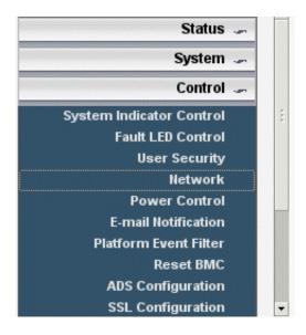
FIGURE 2-4 Embedded LOM Control Menu
